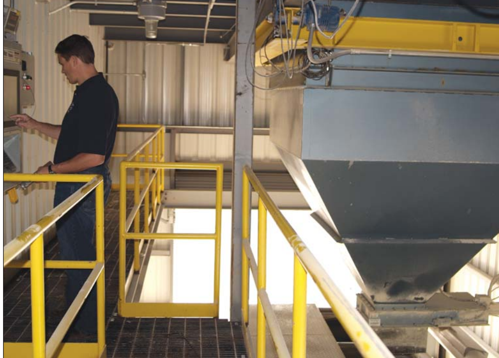
Russ Vering utilizes a Repete loadout interface to load a predetermined quantity of finished feed onto a truck.
