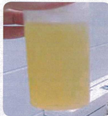
Fuel at cold filter plugging point
